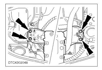
**₾** 11. Remove the left and right-hand radiator support (four bolts).
