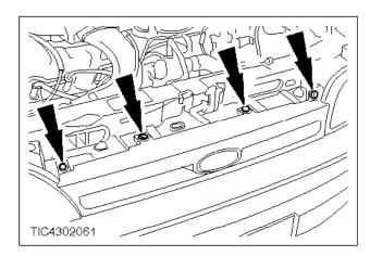
C 1. Remove the Torx retaining screws (four screws).
