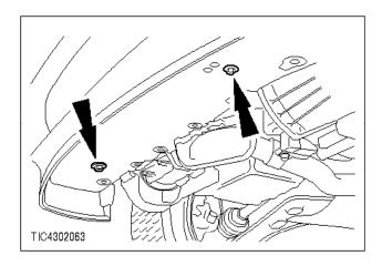
**c** 9. Remove the splash shield nuts.
