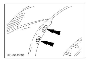
**C** 12. Remove the bumper retaining screws from the left and right-hand wheelhouse.
