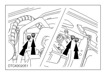
**○** 14. Remove the bumper retaining nuts (four nuts).
