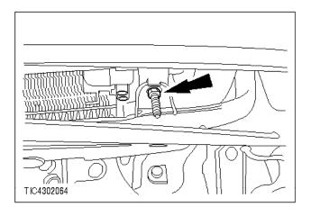
**C** 10. Carefully prise down the splash shield and remove the nuts (one each side).
