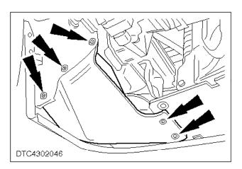
**c** 6. Remove the left and right-hand lower wheelhouse liner extension (five screws each side).
