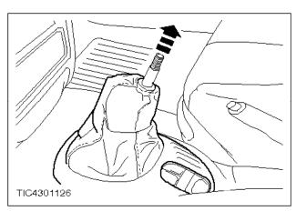
2. Carefully prise up and remove the gear lever gaiter and surround.
