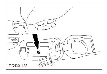
Raise the cassette/storage box lid and remove the rear console retaining screw. 9.
