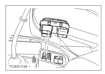
**4**. Disconnect the multiplugs and remove the switch assembly.
