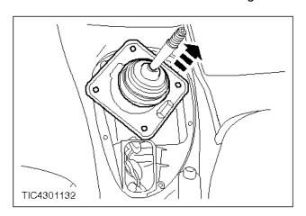
**c** 8. Remove the gearshift floor gaiter and retaining plate.
