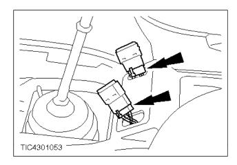
Disconnect the multiplugs and remove the switches.
