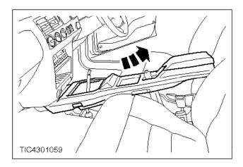
**C** 10. Lift the centre console from the rear and remove.
