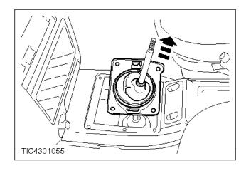
• 6. Remove the gearshift floor gaiter and retaining plate.
