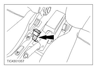
**©** 8. Disconnect the multiplug and remove the switch.
