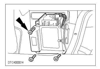
**C** 3. Remove the three Torx retaining bolts and support the module.
