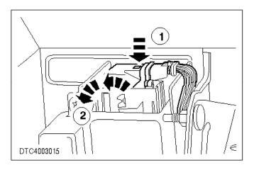
**4**. Disconnect the electronic control module multiplug.
