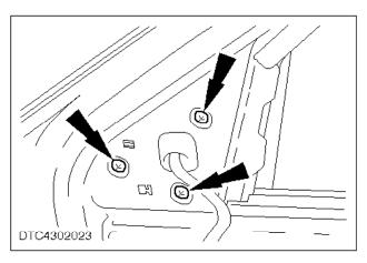
• 6. Remove the three door mirror retaining screws.
