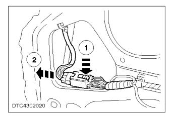
3. Disconnect the electrically operated door mirror multiplug.
