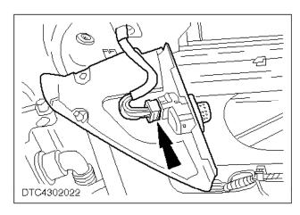
• 5. Disconnect the remote door mirror switch multiplug and remove the mirror inner trim panel and switch assembly.
