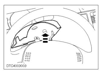
**c** 2. Remove the upper steering column shroud.
