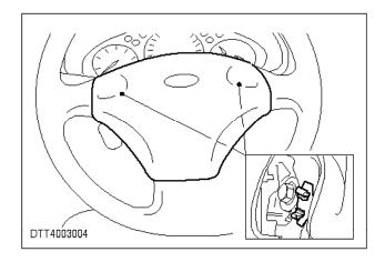
**4**. Ease the air bag module out of the steering wheel far enough to access the air bag module multiplug (two clips).
