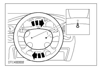
**c** 3. Remove both of the air bag securing bolts.
