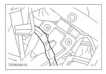
• 6. Unclip the air bag wiring loom from the air bag assembly.
