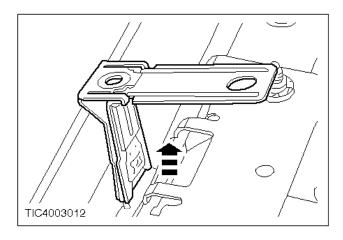
• 9. Ease the bracket out of the assembly.
