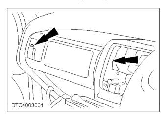
**◆** 3. Working though the vent apertures, remove the air bag module assembly retaining nuts.
