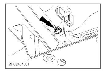
**C** 3. Open the drain valve to drain the coolant.
