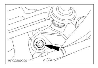
**○** 8. Refit the pulsed secondary air injection pipe assembly support bracket retaining nut.
