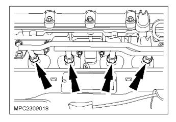
• 7. Loosely assemble the four pulsed secondary air injection pipe assembly unions to the exhaust manifold.
