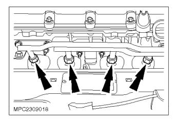
**C** 2. Unscrew the four pulsed secondary air injection pipe assembly unions from the exhaust manifold.
