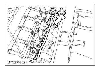
**c** 6. Renew the pulsed secondary air injection pipe assembly.
