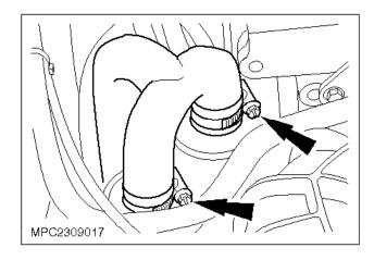
**○** 10. Reconnect the hose from the pulsed secondary air injection pipe assembly (two clips).
