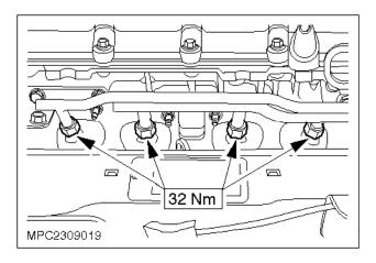
• 9. Tighten the four pulsed secondary air injection pipe assembly unions.
