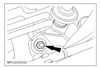
**©** 3. Remove the pulsed secondary air injection pipe assembly support bracket retaining nut.
