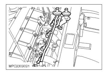
**4**. Remove the pulsed secondary air injection pipe assembly.
