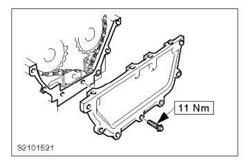
$\mu$  56. Attach the upper timing chain cover (7 bolts).
