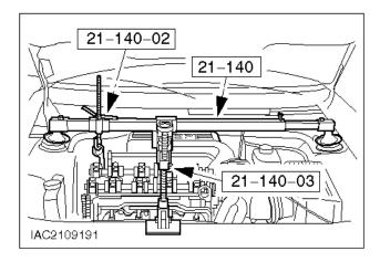
7. Fit the engine support bar.
