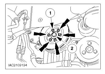
20. Detach the crankshaft pulley/vibration damper.
