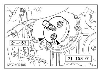
μ 22. Detach the crankshaft pulley/vibration damper hub.
