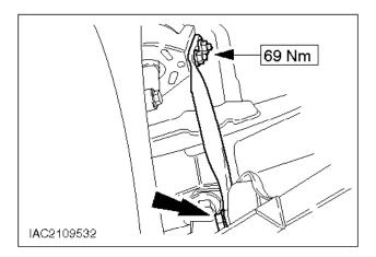
$\mu$  54. Attach the engine mounting brace.
