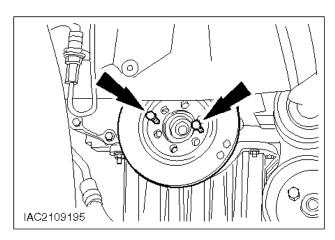
μ 21. Detach the crankshaft pulley/vibration damper (cont.).
