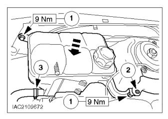
59. Install the coolant expansion tank.
