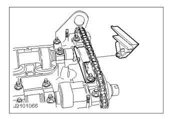
μ 39. Attach the new chain guide rail to the bracket.
