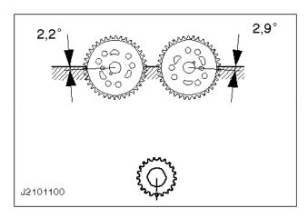
13. Set the camshaft sprockets to the mark.
