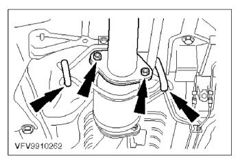
C 7. Detach the exhaust pipe from the catalytic converter.
