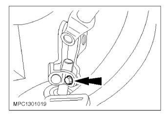
**c** 2. From inside the passenger compartment remove the flexible coupling to pinion shaft pinch bolt.
