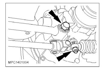
**5** Disconnect the gear change linkage.
