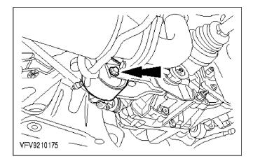
**c** 8. Remove the rear roll restrictor centre bolt.
