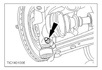
**c** 2. Remove the lower arm to spindle carrier pinch bolt and nut.
