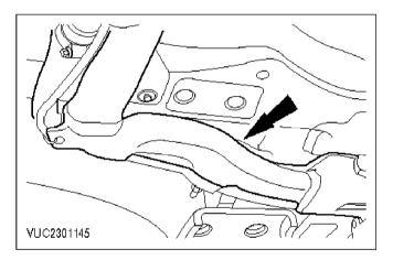
Remove the filler pipe. 11 C
