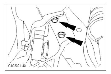
**9** Remove the rear axle bolts.
