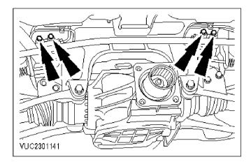
**C** 7. Partially remove the right-hand load apportioning valve (LAV).
