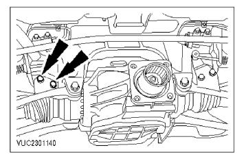
**C** 6. Remove the load apportioning bracket bolts.
