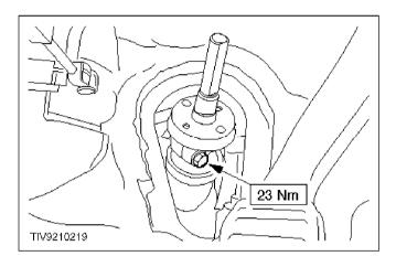
**C** 19 Install the flexible coupling with a new pinch bolt.
