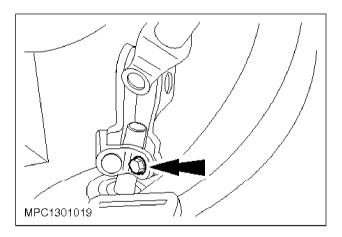
8. Remove the flexible coupling to pinion shaft pinch bolt. C
