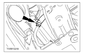
**C** 3. Disconnect the fluid cooler hose.
