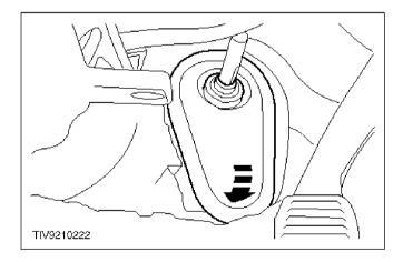
**c** 20 Install the floor seal.
