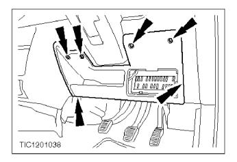
Detach the lower crash pad panel (six screws). 6. C
