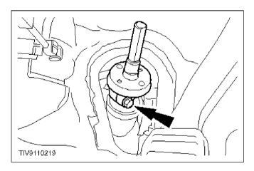
**c** 10 Remove the flexible coupling.
