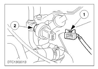
Switch - Pressure - Power Steering - Remove (33 611 0)
