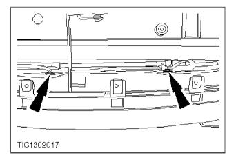
**c** 8. Remove the fluid cooler retaining bolts.
