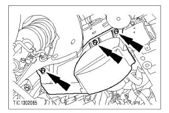
**C** 3. Remove the lower belt guard (three bolts).
