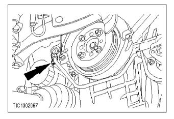
**c** 6. Detach the high pressure pipe securing bracket (one bolt).
