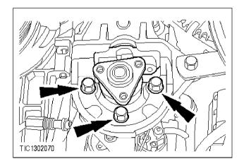
**c** 9. Remove the power steering pump (three bolts).
