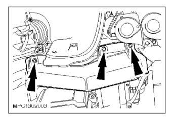
c 2. Remove the lower belt guard (three bolts).
