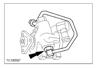
**c** 7. Remove the high-pressure pipe.
