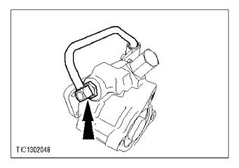
**9** Remove the high-pressure pipe.
