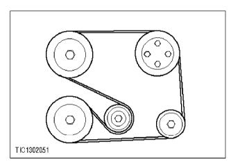
Drive Belt - Power Steering Pump - Install (13 424 0)
