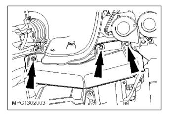
**C** 3. Remove the lower belt guard (three bolts).
