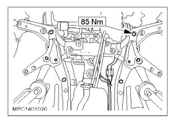
**c** 28. Install the subframe retaining bolts.
