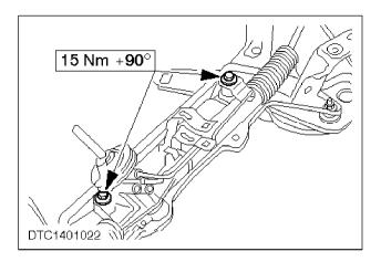
c 26. Install the steering gear.
