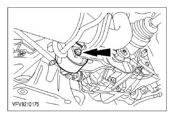
**c** 8. Remove the rear roll restrictor centre bolt.
