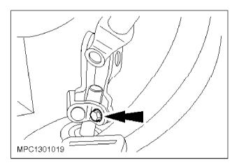
**c** 2. Remove the flexible coupling to pinion shaft pinch bolt.
