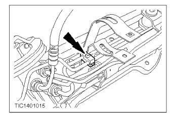
c 18 Disconnect the power steering gear pipes from the clamp (one screw).
