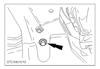
C 17 Remove the engine/transmission mounting bracket lower bolt.
