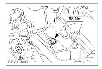
c 43 Install the engine/transmission mounting bracket upper bolt.
