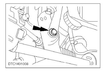
**c** 16 Remove the right-hand engine support bar to subframe retaining bolt.
