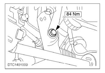
**c** 33 Install the right-hand engine support bar to subframe retaining bolt.
