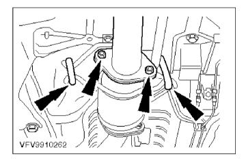
C 7. Detach the exhaust pipe from the catalytic converter and position to one side.
