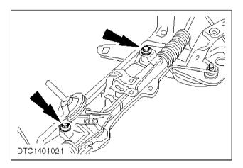
c 24 Remove the steering gear (two bolts).
