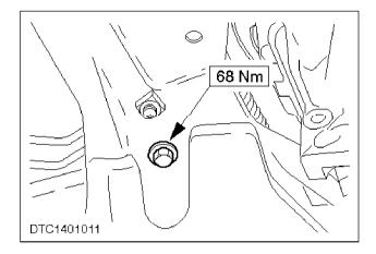
c 32 Install the engine/transmission mounting bracket lower bolt.
