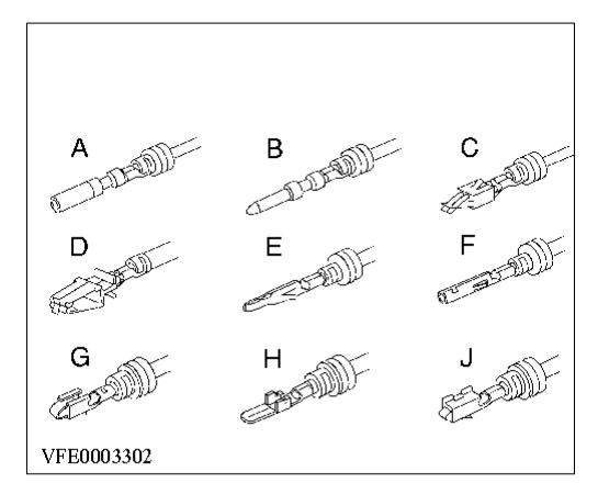
These connectors are already provided with cable terminations of different cross sections. The repair kit also includes various crimp-on sleeves for connection to the loom cable.
