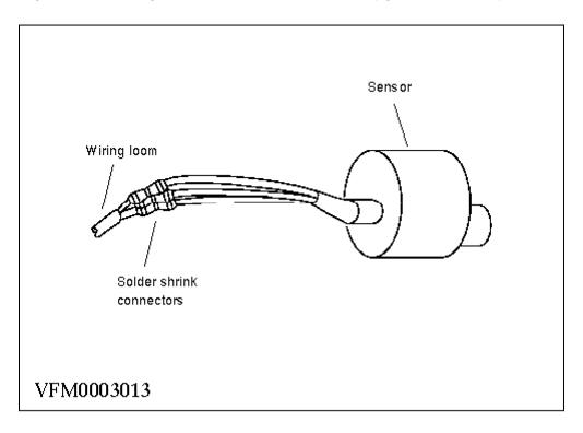
Only solder shrink connectors should be used to attach cut wires together (order from Ford parts). The solder shrink connectors that are available in the wiring loom repair kit from Loewener/Churchill are approximately the same.
