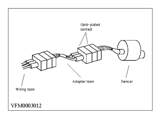
The throttle position sensor (TPS) for 1,1/1,3/1,4/1,6 litre CFI, 2,0 litre EFI and 2,8 litre V6 engines ca
