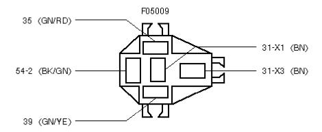
C2253 - B49 Exhaust gas recirculation (EGR) valve position sensor
