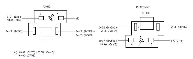
C1505 - N172 Heated seat switch, passenger side
