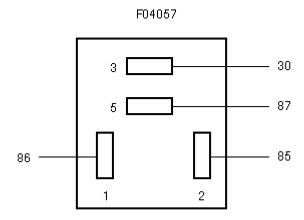
C1170 - K79 Dim-dip relay II, K5 Daytime running lamps relay (DTRL)
