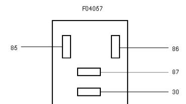
C1163 - K78 Dim-dip relay I, P24 Busbar LHD, K80 Daytime running lamps relay (parking lamps)
