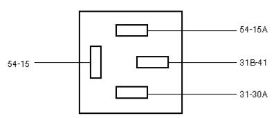
C1167 - K96 Delayed interior light relay, P31 Busbar for interior light w/o delay function
