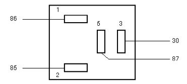
C1161 - K32 A/C Wide Open Throttle (WOT) relay, P30 Busbar for Diesel with A/C
