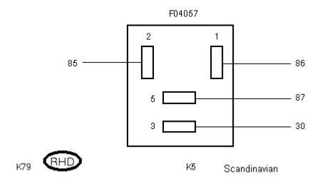
C1171 - A82 Front fog lamp module, P23 Busbar for front fog lamp
