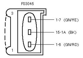
C1922 - P6 Octane adjust plug, P21 Idle adjust plug
