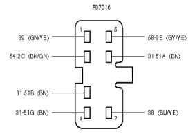
C2281 - M67 Door lock motor, driver's side, M68 Door lock motor, passenger's side
