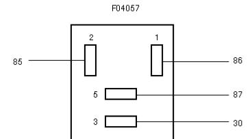
C1174 - K94 Start inhibit relay, P27 Busbar for manual transmission
