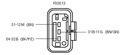
C2256 - D19 Self-test input connector
