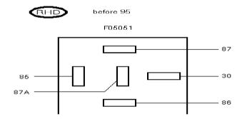
C1157 - K9 Intermittent wiper relay, rear, P25 Busbar for rear window wiper relay
