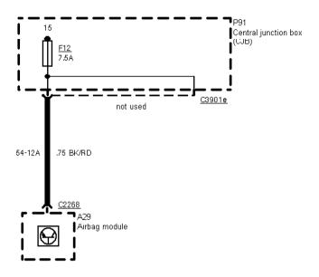
As of 95 without RS Cosworth Diesel/Carburettor models Fuse 13
