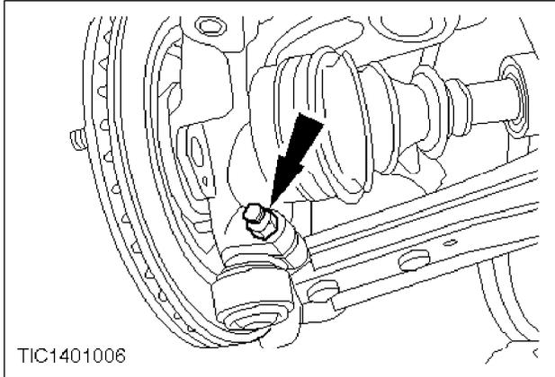
2. Remove the lower arm to spindle carrier pinch bolt and nut.
