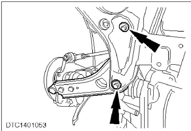
4. Remove the lower arm (two nuts and bolts).
