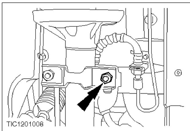
2. Detach the brake hose bracket (one nut).
