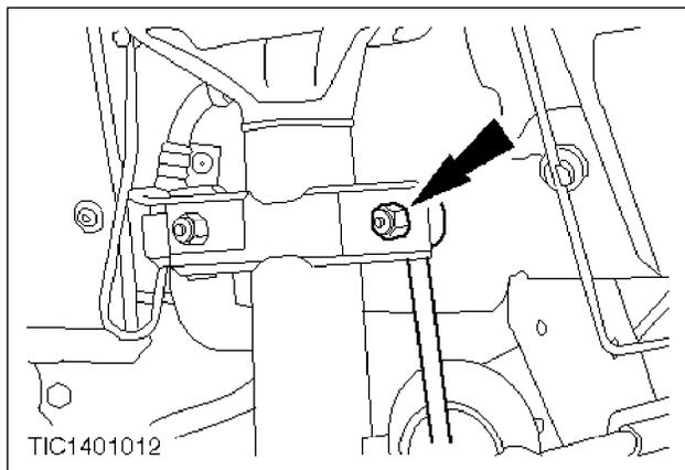
3. Detach the connecting link from the suspension unit assembly (one nut).
