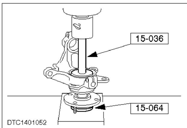
9. Refit the spindle carrier to the hub.
