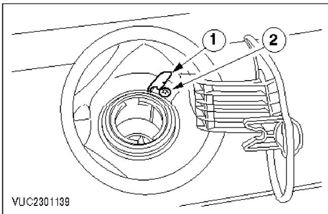
2. Remove the fuel tank filler pipe top retaining screw.
