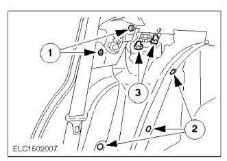
7. Release the upper right and left-hand suspension struts.
